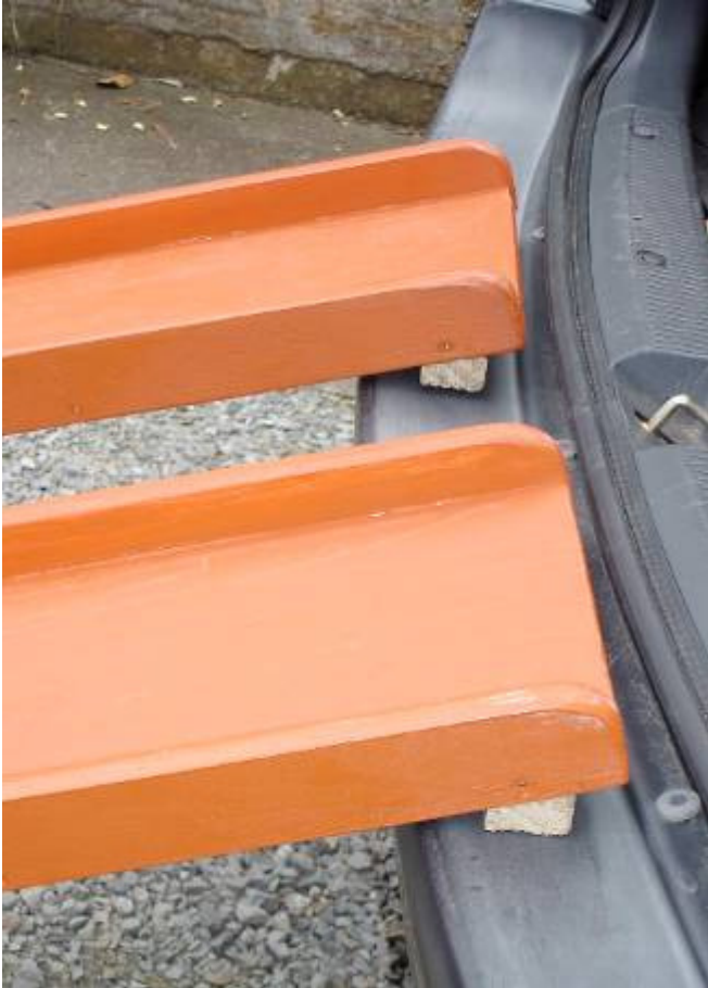
Under-ramp fillets that provide a good footing on the bumper.
