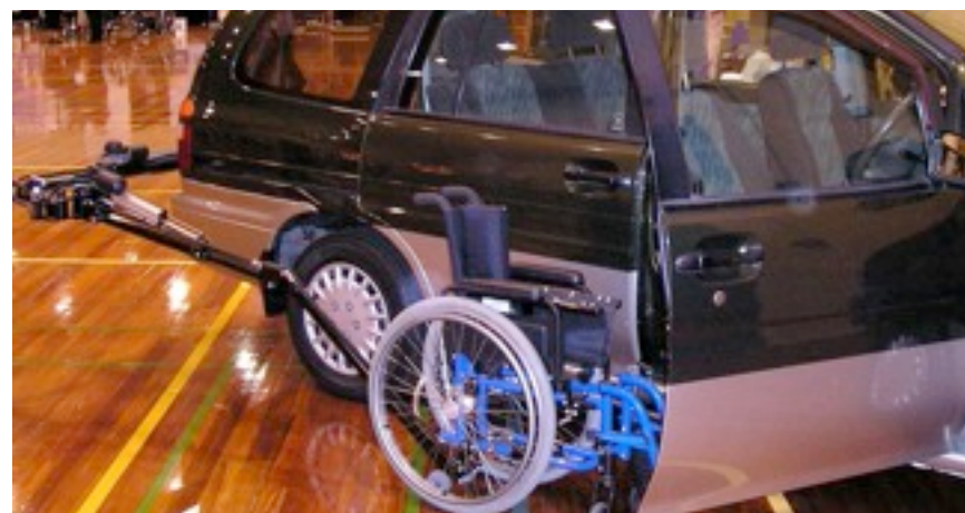
Above, the loader lifts a wheelchair out of a wagon and delivers it to the driver's door. The process is reversed to return the chair.
